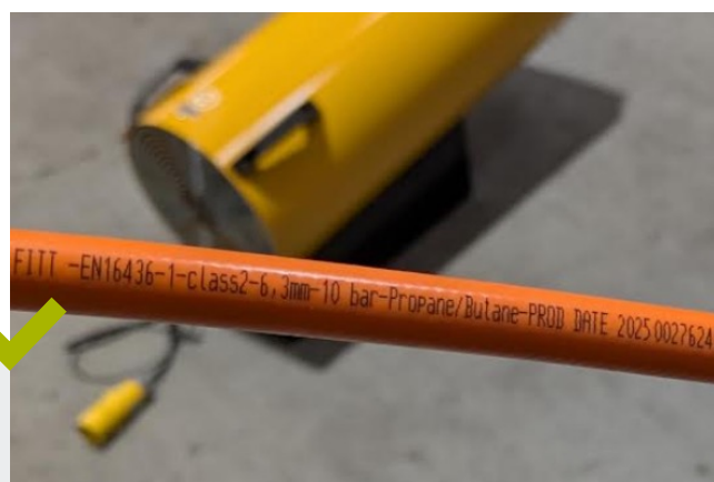
Fig. 2 BS EN 16436-1 Class 2 Within expiry (new) marked with production date.
