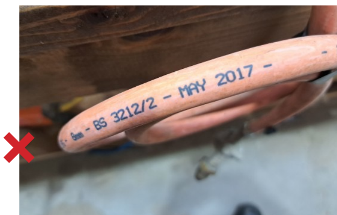
Fig. 1 BS312 Class 2 Expired (Displaying UV degradation) marked with production date.
