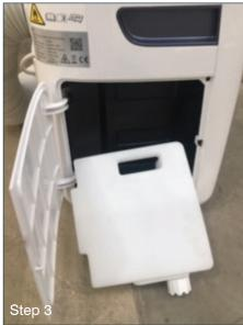
Note: Step 3 will only be necessary to keep the coils/veins and condensate trays free of contaminants or otherwise where this is necessary to satisfy the requirements of the client for example where the equipment is to be used in Healthcare environments.
