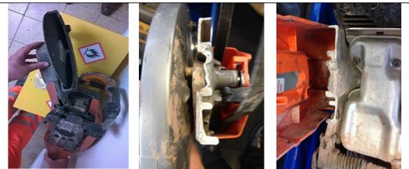
Cracking / fracture has occurred at the crankcase casting where the drive head (aka bearing housing) is attached.
