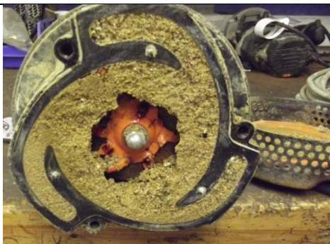
Sub-Pump – debris and a destroyed impellor 50mm pump, sewage waste contaminating pump
