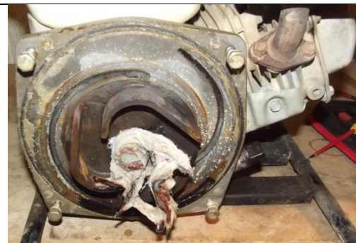
Sub-Pump – debris and a destroyed impellor 50mm pump, sewage waste contaminating pump
