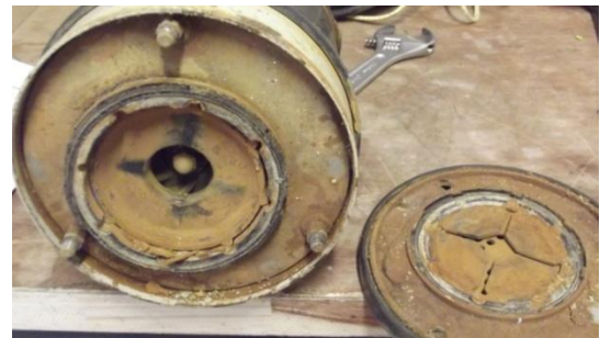
Sub-Pump – debris and a destroyed impellor 50mm pump, sewage waste contaminating pump
