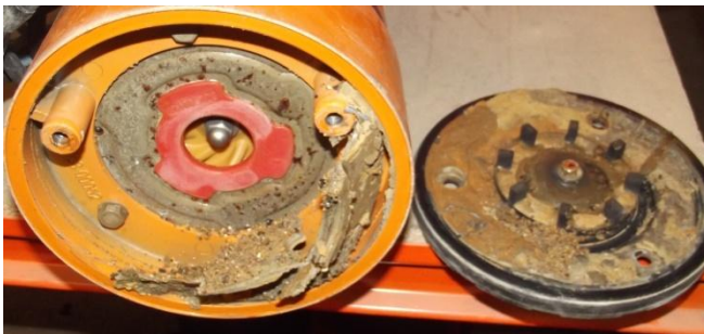
Sub-Pump – debris and a destroyed impellor 50mm pump, sewage waste contaminating pump
