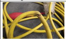
**6 – Cable Profile**Thickness of insulation is critical for cable performance – wear to sheath will affect its performance
