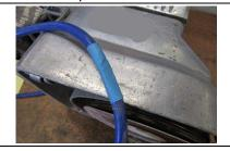
**5 – Cable Damaged**Obvious wear to extension cable
