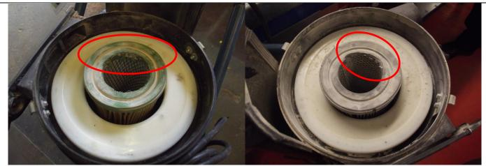
Primary / Outer filter – heavily contaminated – reverse pulse cleaning has not been completed during hire / at service. Filter life is in excess of 12 months if serviced correctly Note: Washable filters are available.
