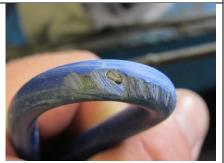
6 -Incorrect wiring - trapped between frame and cover
