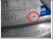
5- Top cover cracked / broken replace
