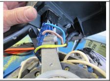
9 - Poor plug wiring / fuse clip loose - see Tech Bulletin 8
