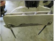
**5** – Socket damaged on Clare A255 – repair required
