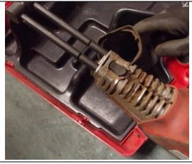
Adjustable foot mechanism retaining bolt loose (circled)
