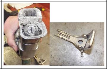
Screws – have been loose, missing and / or incorrect for application
