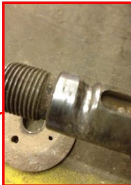
Dismantled drive flange assembly showing hidden damage
