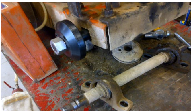
Repaired - New shaft / nut, bearings, and flanges.
