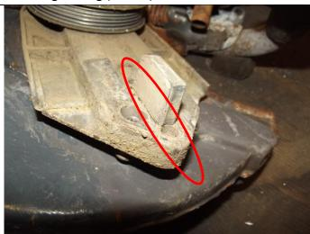
Cracking affects the drive head casting - known as bearing housing by the manufacturer. To fully inspect, remove the drive head. Cracking may also be visible by removing the inner retaining bolt and inspecting the threads of the casting for cracking using a suitable torch.
