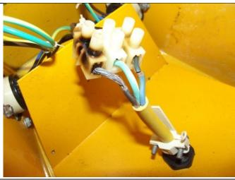
Transformer internal corrosion, heat damage to circuit breaker, cracked casing and low durability 240v plug fitted
